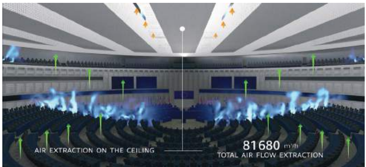
CFD modeling of European parliament showing correct extraction of potential pollution in auditorium with lower performances in balconies.
